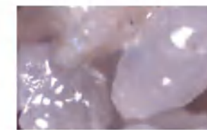
Silica sand binder coating method 60x enlarged image of 0.8mm Grade 4 silica sand
